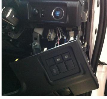
50. Due to CANBUS wiring system on vehicles fitted with LED headlights, there is no usable power supply/signal for the bullbar clearance lights on the connector at the head lamps.
