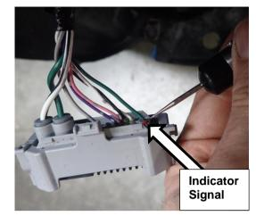
52. Using supplied scotch locks, connect the LED Indicator/clearance light looms as per table.
