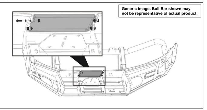
37. Fit the number plate bracket to the top face of the lower-centre pan on the bar using 3 x M6 x 20 hex bolts, flat washers and flange nuts.
