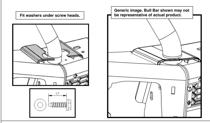
47. Attach the buffers to the front face of the bar using the angled cup washers, flat washers and screws.
