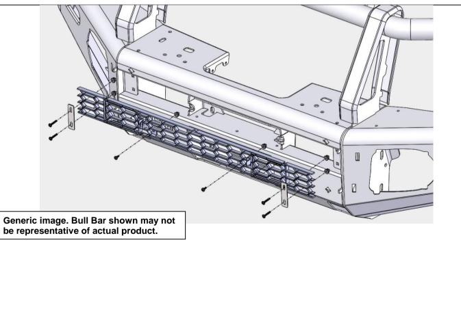
46. Place each of the Top Buffer sections onto the bar as shown. Ensure that the buffers are keyed together correctly. Fit 5 x screws and washers. Do not tighten screws. Leave enough play in buffers for adjustment later.
